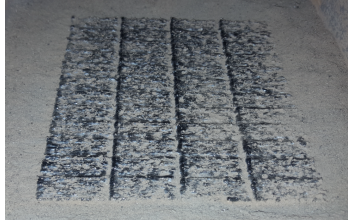
Figure 4: 120 × 120 mm sintered crust produces on LHS-1 simulant.
