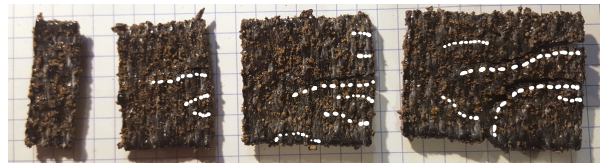
Figure 6: Development of cracking as the width of a 30 mm long tile is increased from 10 to 40 mm. Cracks are highlighted by dotted white lines under the cracks.
